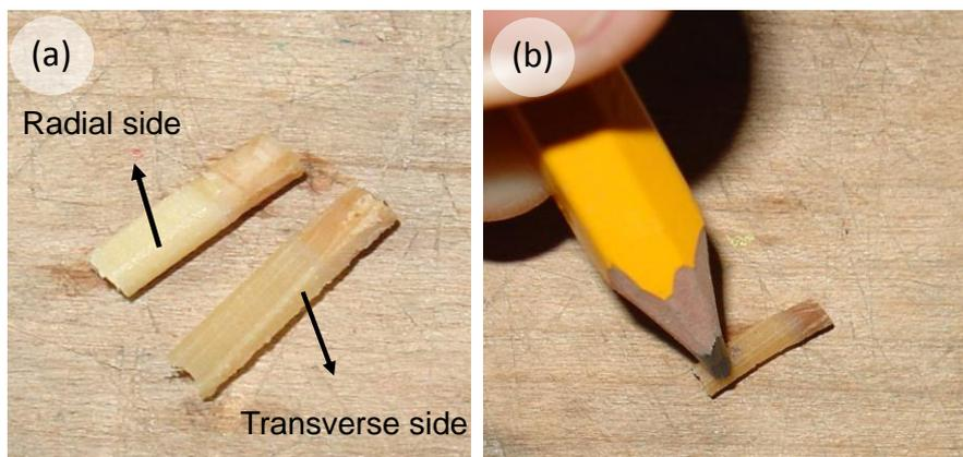
**Figure 2:** The transverse plane of the microcore is identified (a) and marked with the pencil (b)
