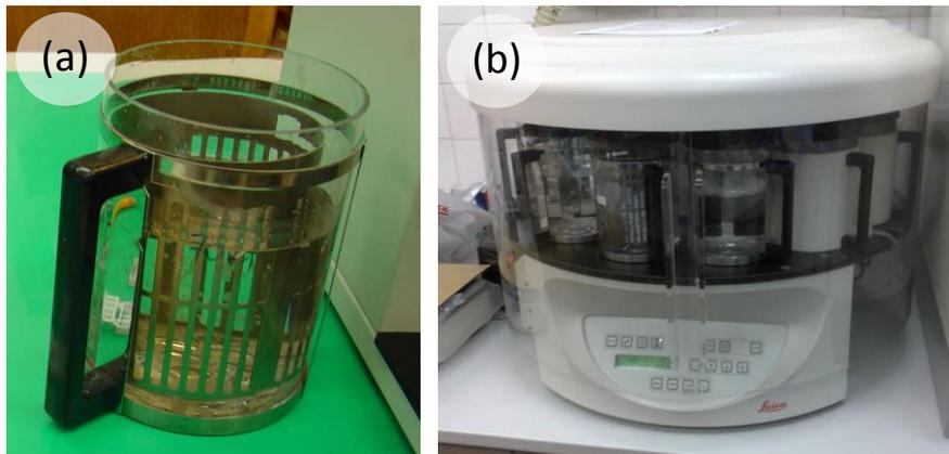
**Figure 3:** The prepared samples are placed into a basket of the tissue processor (a). The tissue processor contains twelve vessels/containers filled with different concentrations of Ethanol, clearing solvent and paraffin (b).
