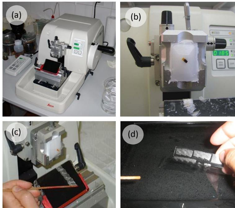
**Figure 5:** Samples are cut with a rotary microtome (a). Before sectioning, the paraffin blocks are trimmed to remove excess paraffin and level the surface (b). Sectioning is performed (c) after the trimmed samples were placed for at least two hours into water. The formed ribbons should be transferred into warm water (40° C warm) to stretch them. Sections are then transferred to the object glasses (d).
