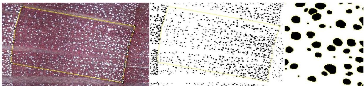
**Figure 3.** Stages in the analysis of wood anatomy, using „ImageJ“ program.
