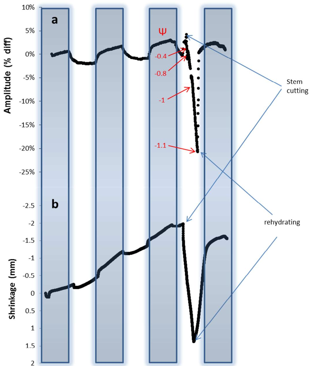
**Figure 3-** Monitoring grapevine petiole water status through continuous NMR (a) and dendrometer (b) measurements for three consecutive days. Stem cutting, and its rehydration through submergence in water were imposed to simulate water stress and its alleviation. Leaf water potential values (red) were taken after the stem cutting.
