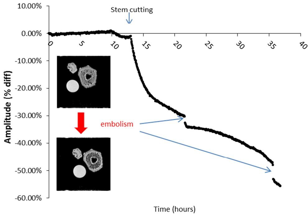
**Figure 2-** Stem dehydration (due cutting of its roots) monitored with portable NMR. Large embolism events, (marked in the image) were inflicted by cutting the stem 15cm and 2 cm below the measured spot, thus allowing air to penetrate the vessels (As also demonstrate by the MRI images in a stem and a petiole).
