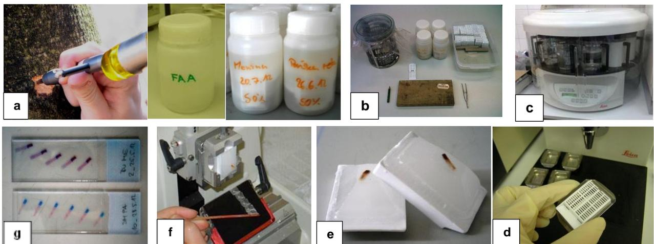
**Figure 1** Practical micro-coring method application. (a) Field sampling of micro-cores, (b) Sample preparation, (c) Dehydration and paraffin infiltration, (d) Paraffin embedding, (e) Paraffin block trimming, (f) Cutting procedure, (g) Finished slides with cross-sections of spruce and beech.
